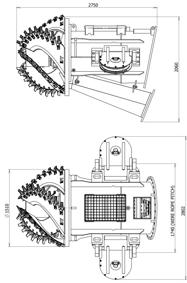
LADDER PIPE FLANGE: DN1000 28 x Ø36 HOLE AT P.C.D.
